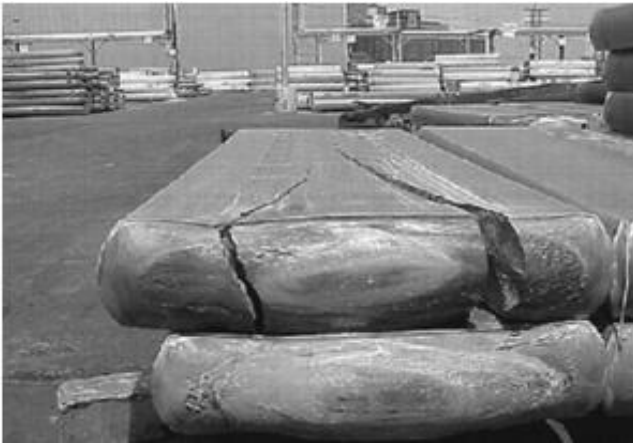
Fig1. Cracking in the cast aluminium ingot due to excessive residual stress [1].
