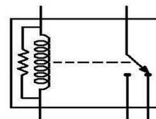
A relay is a switch which is operated by electricity. It is usually electromagnetic device which has coil. When this coil is supplied with power, a magnetic field created and will operate mechanical switch. There are solid state relays which do not have moving parts but are very expensive compared to small mechanical relays. Pictures in this page shows typical small electro mechanical relay. Relay is used when we need to handle high voltages and currents through microcontroller operated system.
