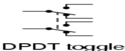
of contacts can be in one of two states: either "closed" meaning the contacts are touching and electricity can flow between them, or "open", meaning the contacts are separated and the switch is nonconducting. The mechanism actuating the transition between these two states (open or closed) can be either a "toggle" (flip switch for continuous "on" or "off") or "momentary" (push-for "on" or push-for "off") type.
