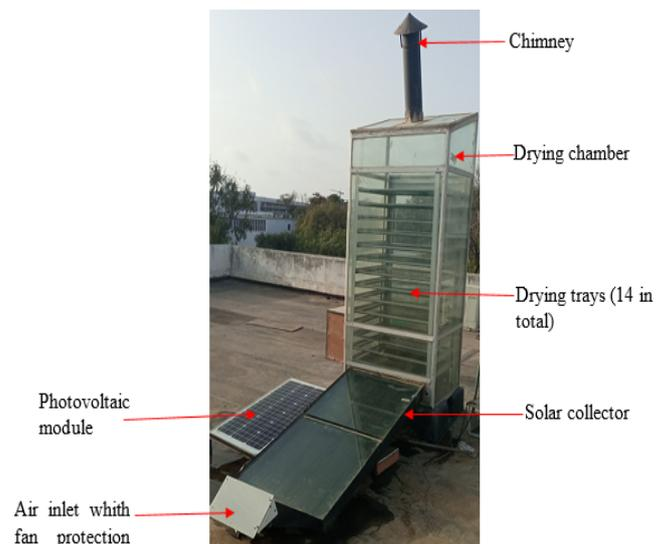
Figure 1: Photograph of the solar dryer
