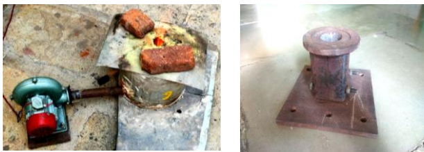
Fig.1 (a) Coal fired furnace (b) Squeeze casting Split Die
