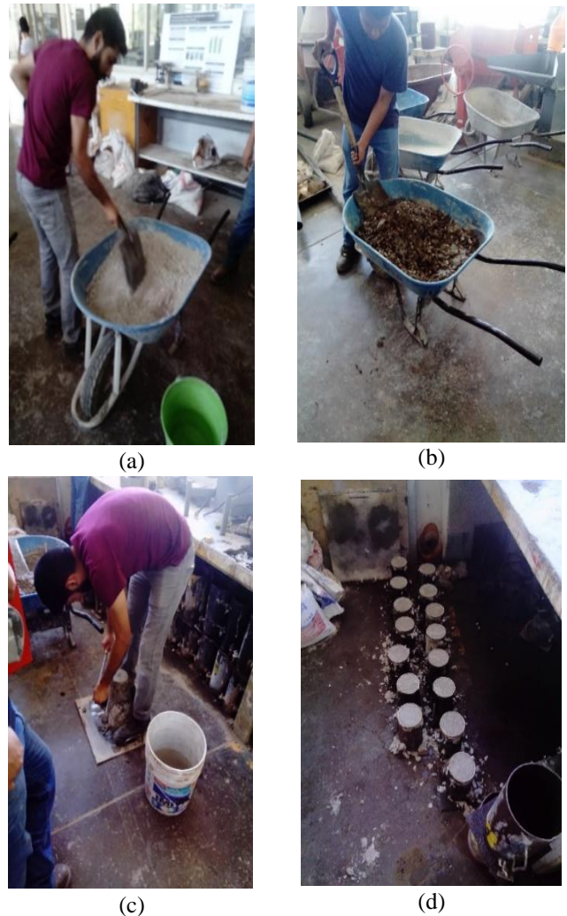
Fig. 3- Preparation of the standard mix (a) preparation of materials, (b) mixing of materials, (c) slump test and (d) preparation of cylindrical samples. Own elaboration
