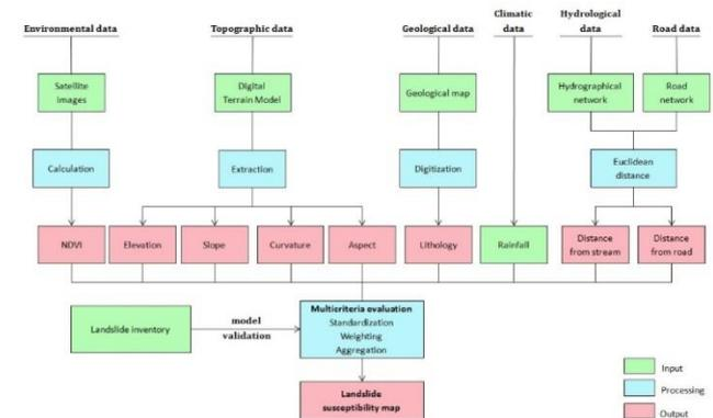
Fig. 2. Flowchart of model construction
