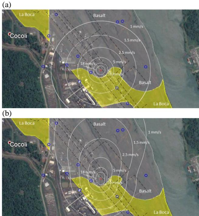
Fig 5: Iso-velocity map from blast#14 with geological domains superposed for (a) traditional analysis and (b) multidirectional analysis.
