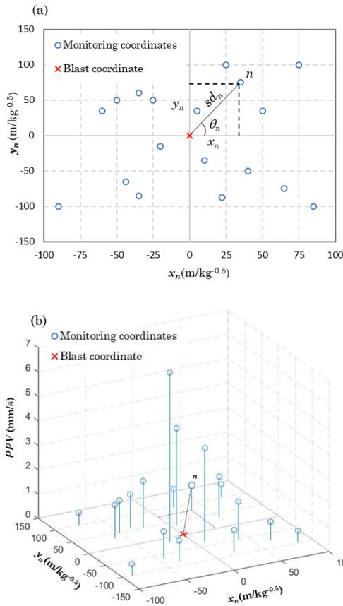
Fig 1: Schematic monitoring and blasting locations at (a) the parametric plane space and (b) with vibration intensities
