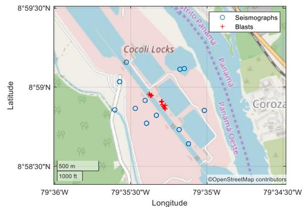
Fig 2: Seismographs and blasts locations for the first 20 blasts in the Panama Canal Expansion Program.
