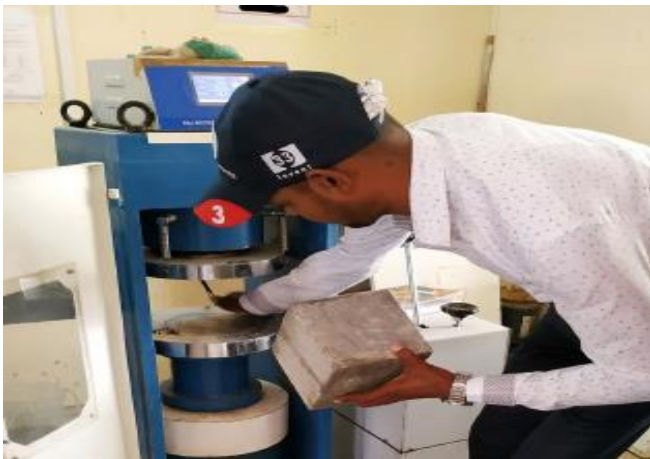
Figure 5: Compressive strength testing using UTM
