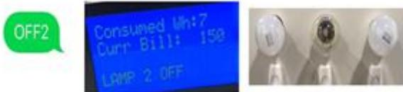
Fig. 11: Switching off the light through SMS
