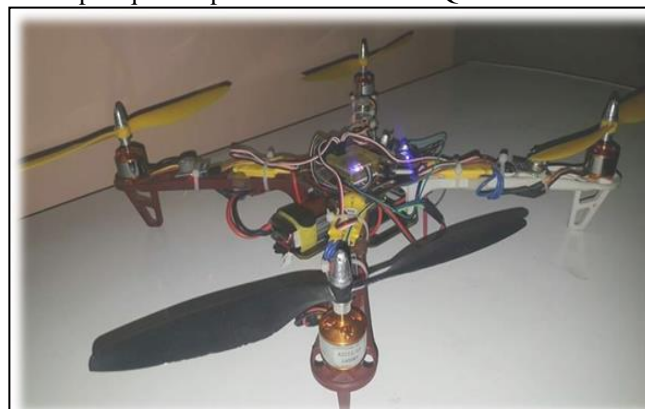
Fig. 3: Final version of the developed quad-copter with set of MQ sensors
