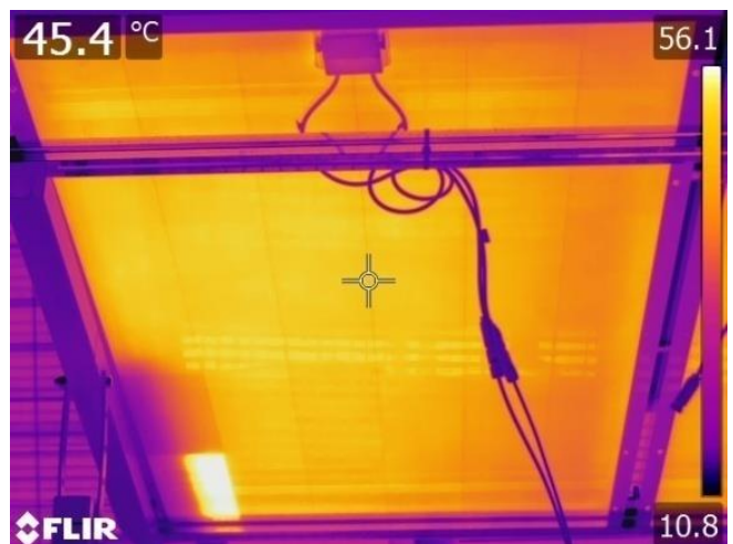
Fig. 4.1. Photo of a partially shielded SV60-255 photovoltaic panel from the back site made by infrared camera.
