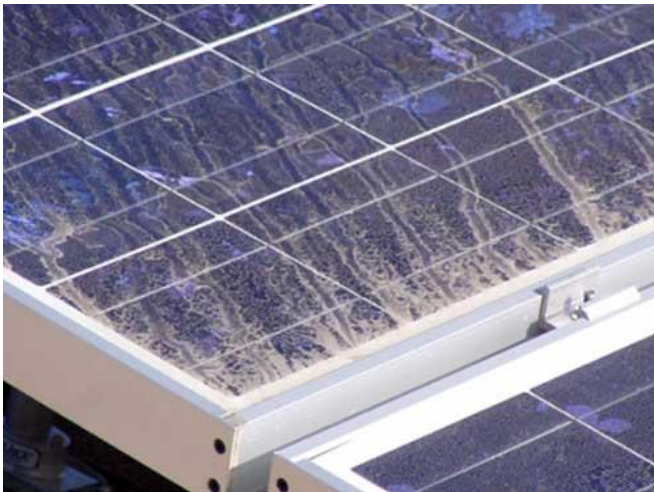
Fig. 3.1. Pollution of the photovoltaic panel
