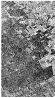
Fig. 4. Airborne SAR image in C band, in horizontal polarization with resolution of 4.6 meters
