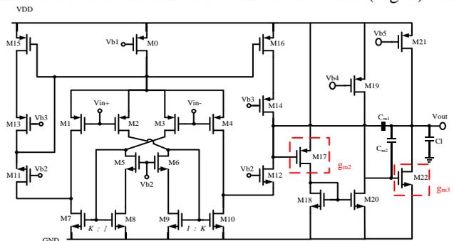
Fig. 2. Improved recycling nested Miller compensation (IRNMC) amplifier.
