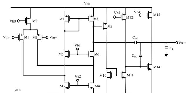
Fig. 1. The conventional nested Miller compensation (NMC) amplifier.
