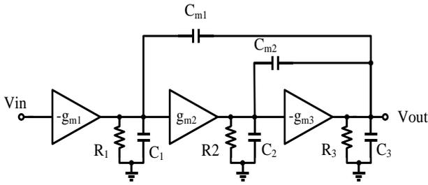
Fig. 3. Signal representation model of IRNMC amplifier.
