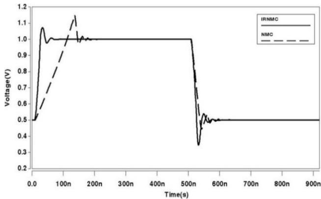
Fig. 5. Transient responses of amplifiers with a 100pF//1kΩ load.
