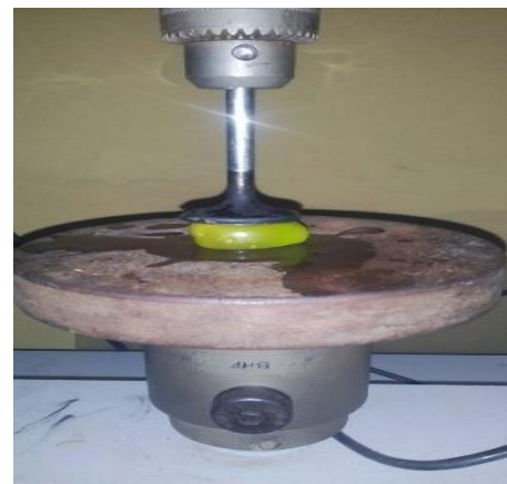
Figure 1: Gmelina fruit undergoing compression testing (Longitudinal loading orientation)
