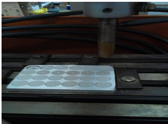
Fig. 6 The machined work piece specimens.
