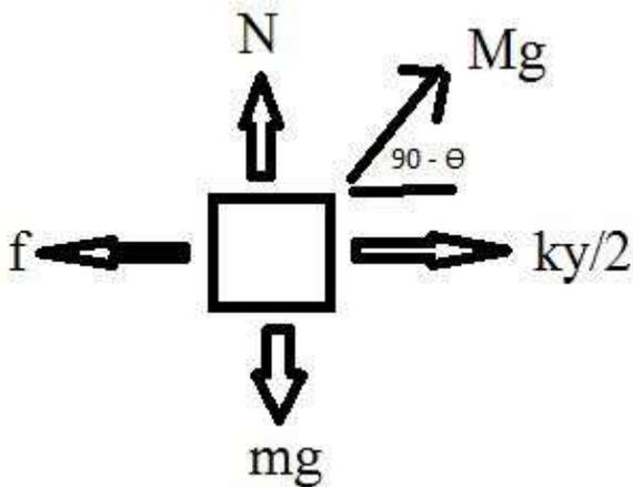
Here  $M$  is mass of the shield. According to figure of system description it will act at an angle  $\Theta$  with the horizontal.
