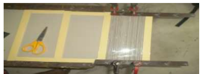
Fig.2.2.2(c) Composite at curing
