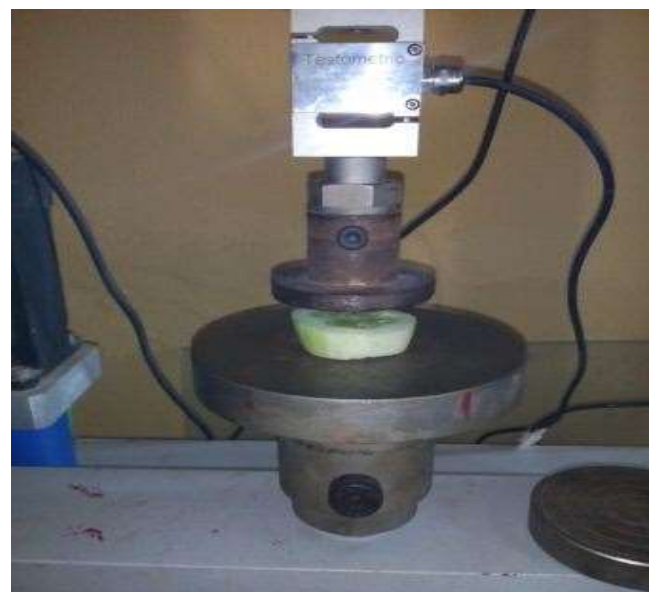
Plate 1: Cucumber fruit undergoing quasi compressive test using Universal Testing Machine (Testometric model, series 500-532)
