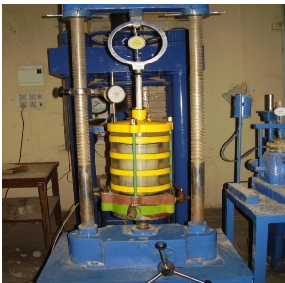
Plate 2. Large triaxial test–Experimental set up
