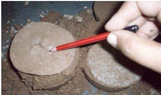
Plate.3. Rupture failure of fabric reinforcement
