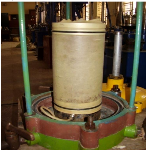
Plate 1. Soil specimen preparation and test set up for triaxial testing.
