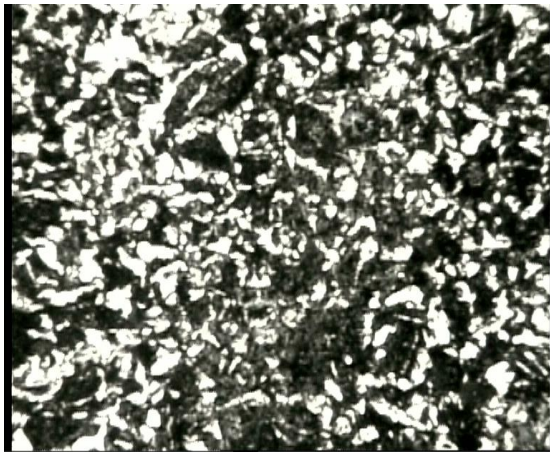
Fig 5: heat affected zone by using mild steel filler and mild steel electrode
