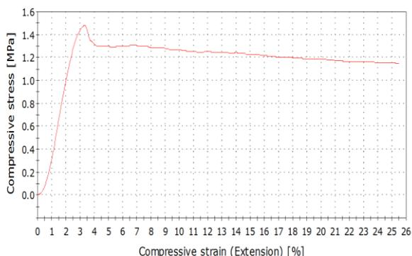
Fig. 3: Compressive stress-strain curve for carbon fibre laminate composite.
