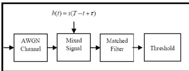
Figure3 Block Diagram of Matched filter detection
