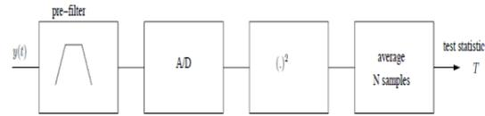
Figure 4 Block diagram of an Energy Detector. [26]
