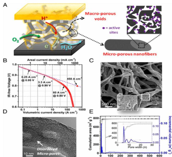
[A] A schematic drawing of macro-pore–micropore morphology and charge/mass transfers in the nanofibrous network catalyst at the fuel cell cathode.
