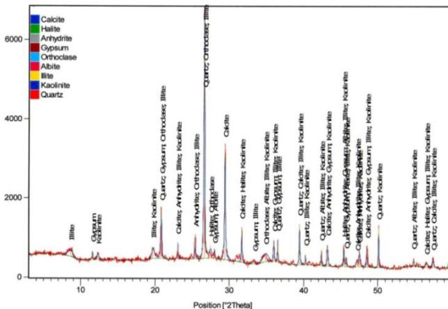
Fig.1. Mineralogical analysis of bricks in earth of the walls of the ksour
