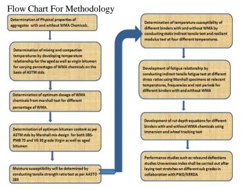
Physical properties of aggregates SBS-PMB70 and VG30 Grade for virgin as well as aged bitumen are to be determined with and without WMA chemicals.
