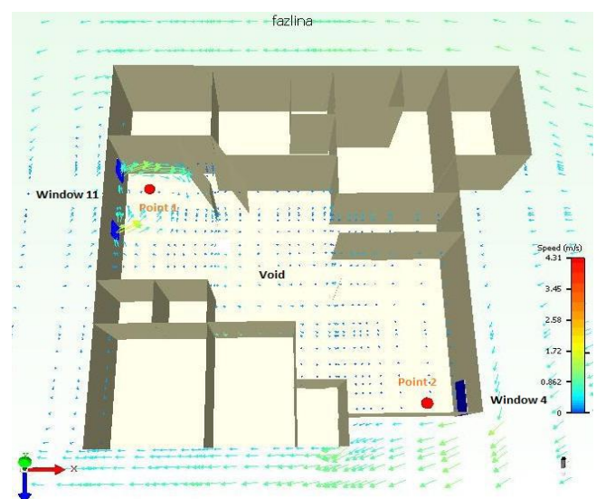
Fig. 14. Predicted wind vector in the house at Ground Floor in Condition 1, night time.
