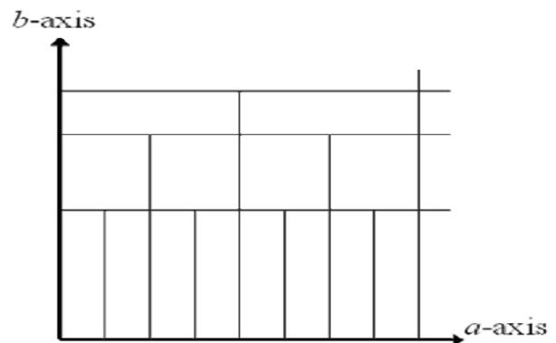
**Fig .3 Time-frequency resolution plane for wavelet transform.**
