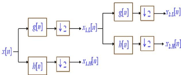
Fig.5. Multi-level 1-D discrete wavelet transform
