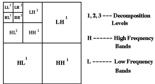
**Fig.2 DECOMPOSITION BY DWT:-**
