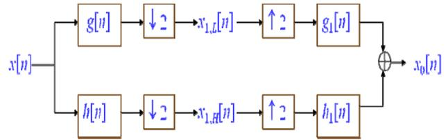
Fig .6 the block diagrams of DWT and IDWT.
