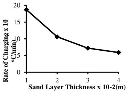
Fig. 5 Rate of Charging Sands at Different Sand Layer Thicknesses.
