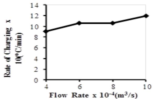
Fig. 4 shows the influence of flow rate on the rate of charging sand. It was noted that the rate of charging sand increased slightly as the flow rate increased.
