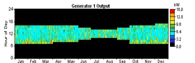
Figure 22 Generator Output of PV-Diesel-Biodiesel Hybrid System.
