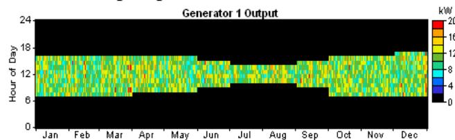
**Figure 15** Generator Output During Sunshine Hours.
