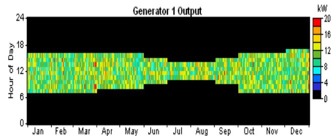
**Figure 15** Generator Output During Sunshine Hours
