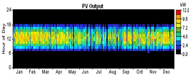
Figure 17 PV Output of PV-Diesel Hybrid System.
