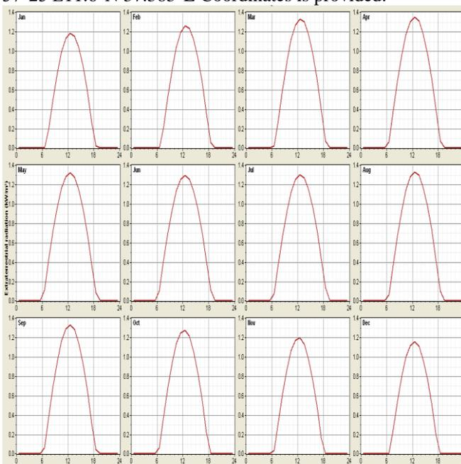
Figure 5 Extraterrestrial Horizontal Radiation Daily profile
