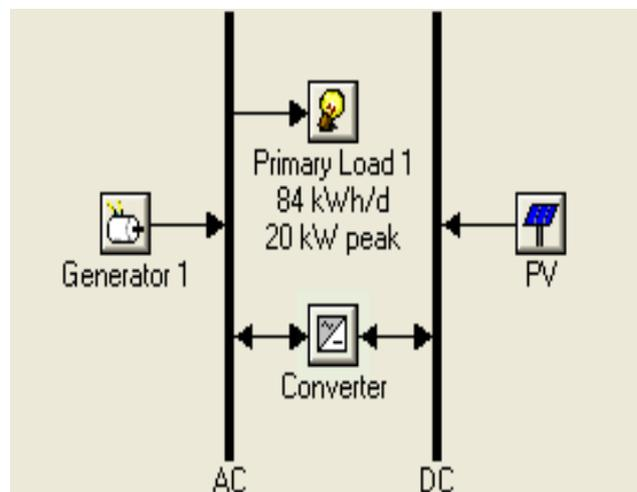
Figure 3 Equipments Considered in Homer Simulation
