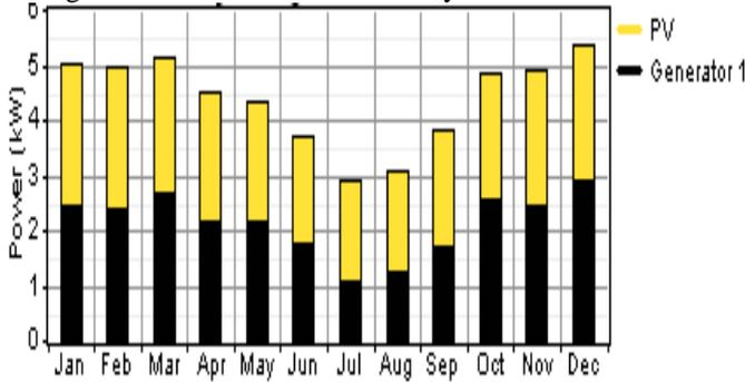
Figure 16 Monthly Average Electric Production by PV-Diesel Hybrid System.
