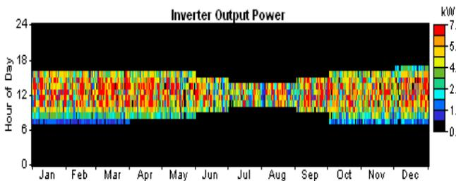
Figure 19 Inverter Output of PV-Diesel Hybrid System.
