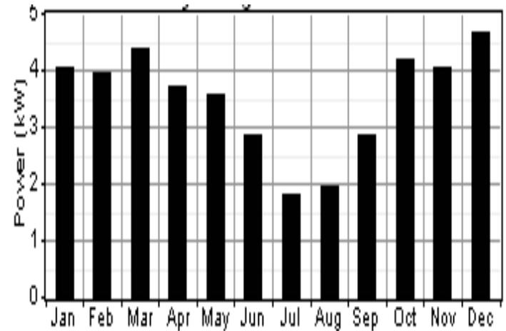
**Figure 0-1** Monthly Power Production by Diesel Generator in B20 Powered System
