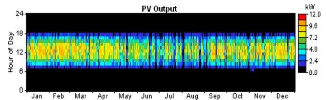
Figure 21 PV Output of PV-Diesel-Biodiesel Hybrid System.
