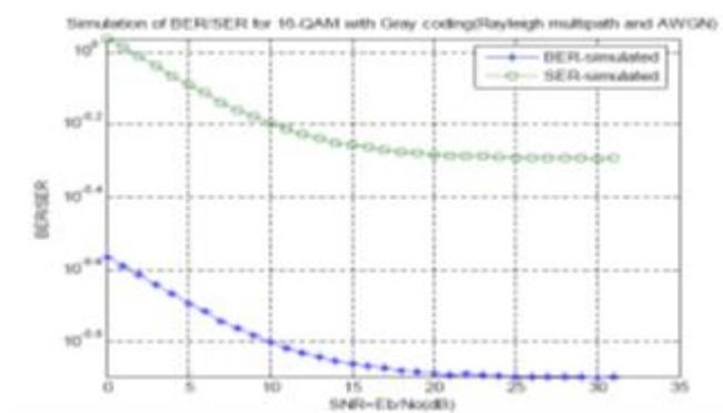
Fig. 9: Performance Comparison of 16-QAM in W-CDMA system.
