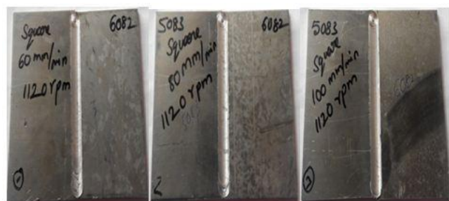
(b) Weld joints fabricated with Square tool pin profile
