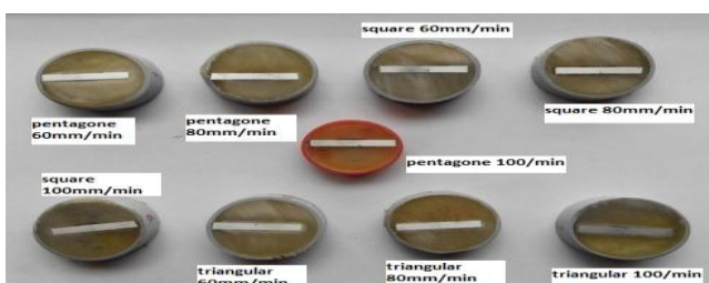
Fig 7. Moulds prepared for metallographic study
