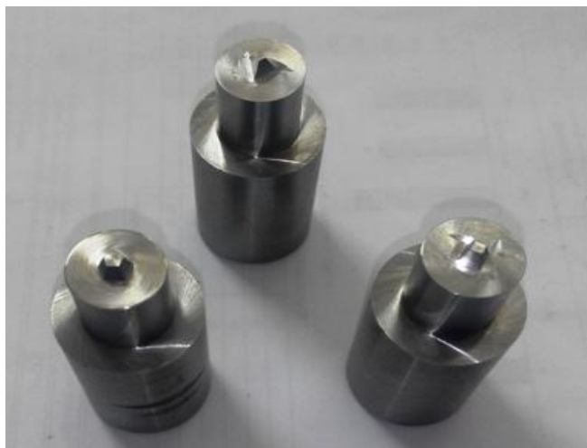
Fig 2. FSW tool pin profiles
