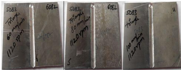
(c) Weld joints fabricated with Triangular tool pin profile
