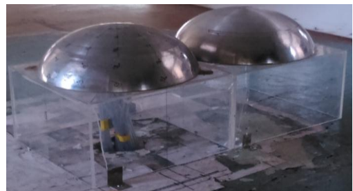
Fig. 5 Model of rectangular plan building with 2 domes
