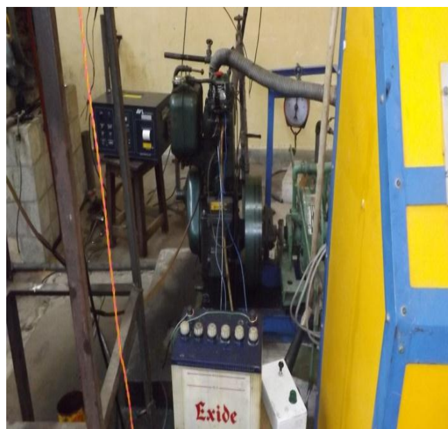
Fig1.1 Experimental setup of GHSI LHR Engine Test rig
