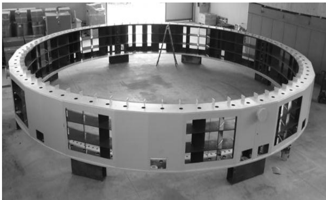
Fig. 2: Fabricated Stator Casing.
