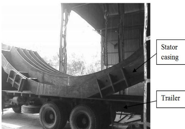
Fig. 5: Stator casing loaded on a trailer without core and winding.
