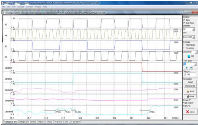
Fig.19 Post-Layout Simulation (Voltage vs. Time) of 2-bit comparator (Configuration 1) in 45nm using GDI/AVL Technique
