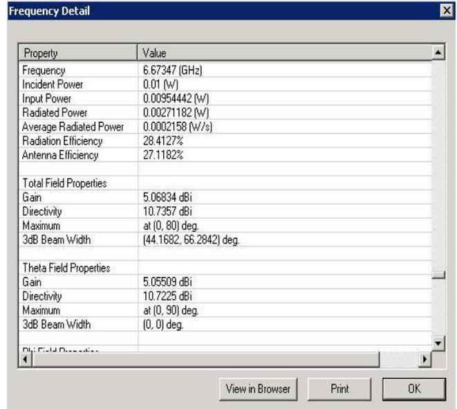
**Frequency detail at 6.6734 GHz of third iteration for D.S. fractal antenna**
