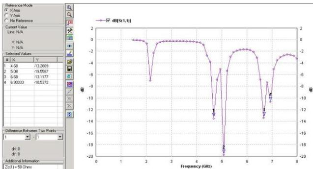
**Figure 11 - Return loss Vs frequency plot of D.S. third iteration**
