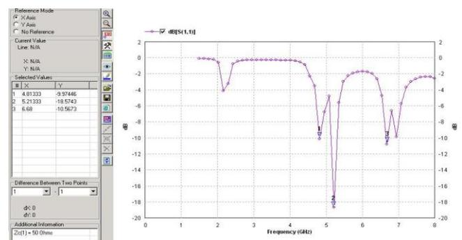
Figure 7- Return loss Vs frequency plot of first iteration for D.S. fractal antenna
