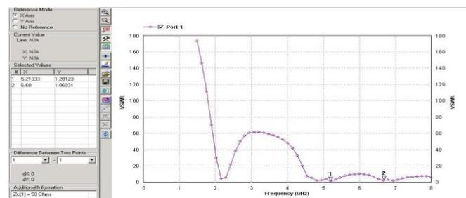
Figure 8 - VSWR of first iteration for D.S. fractal antenna
