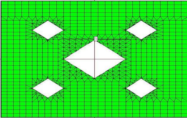
Figure 3- Second iteration for D.S. fractal antenna
