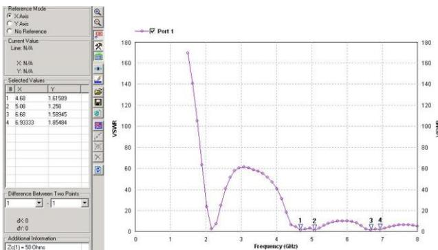
**Figure 12 - VSWR of third iteration for D.S. fractal antenna**
