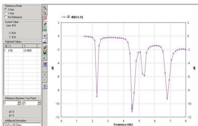
Figure 5- Return loss Vs frequency plot of base shape for D.S. fractal antenna
