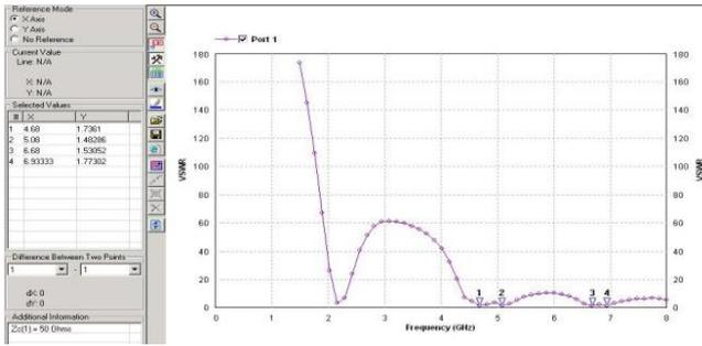
**Figure 10- VSWR of second iteration for D.S. fractal antenna**
