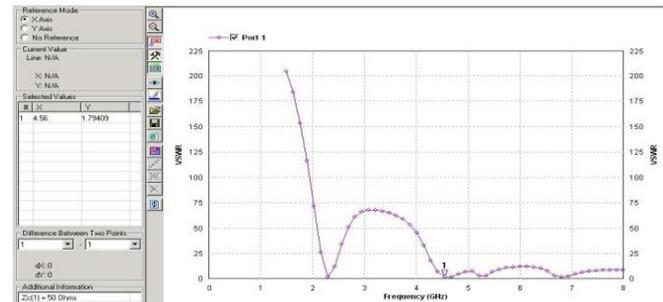
Figure 6- VSWR of base shape for D.S. fractal antenna
