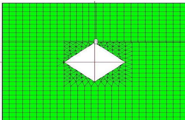
Figure 2- First iteration for D.S. fractal antenna
