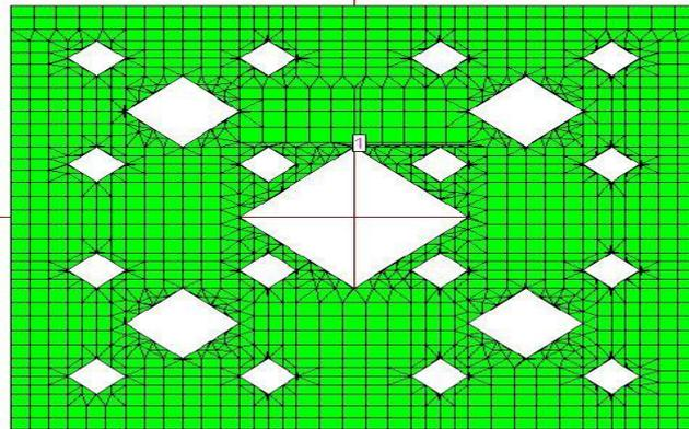
Figure 4- Third iteration for D.S. fractal antenna
