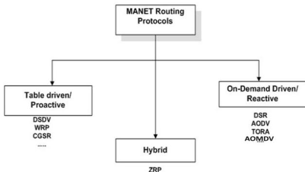
Fig 3.1: Classification of routing protocols
