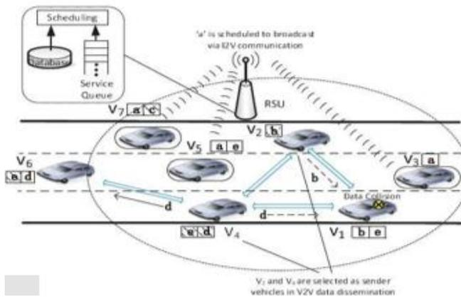
Fig.4.Fog computing in SDN in Vehicular networks
