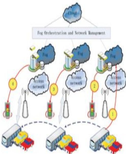
Fig 2.Fog computing in smart traffic lights and connected vehicles.
