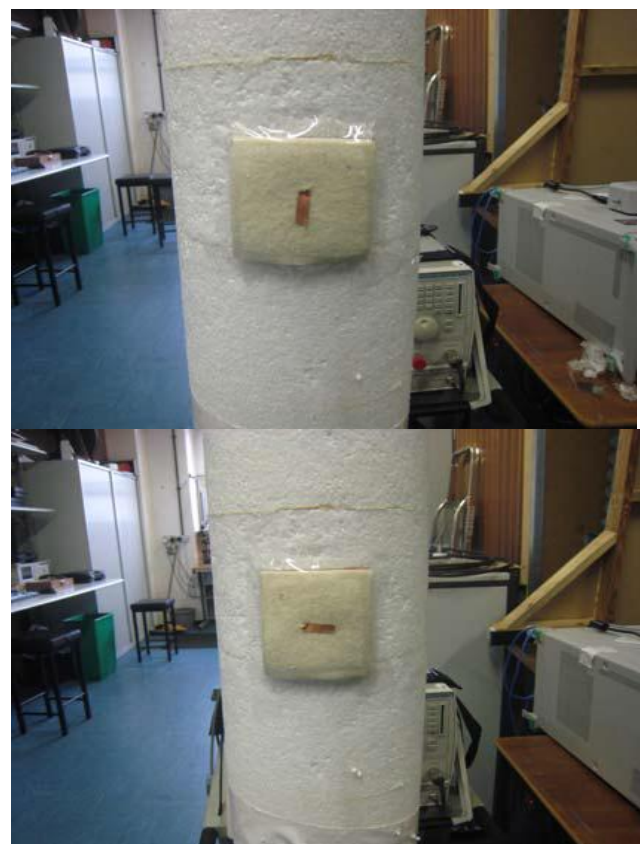
Figure 7. Measurement setup for bending condition. (a) H-plane bending, (b) E-plane bending
