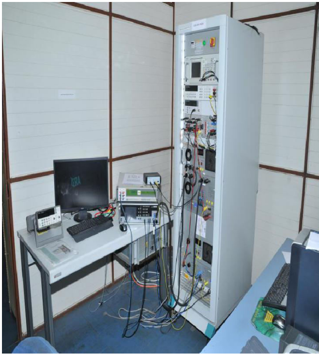
Fig. 2 Calibration of MSB 100 by PPCS Set-up
