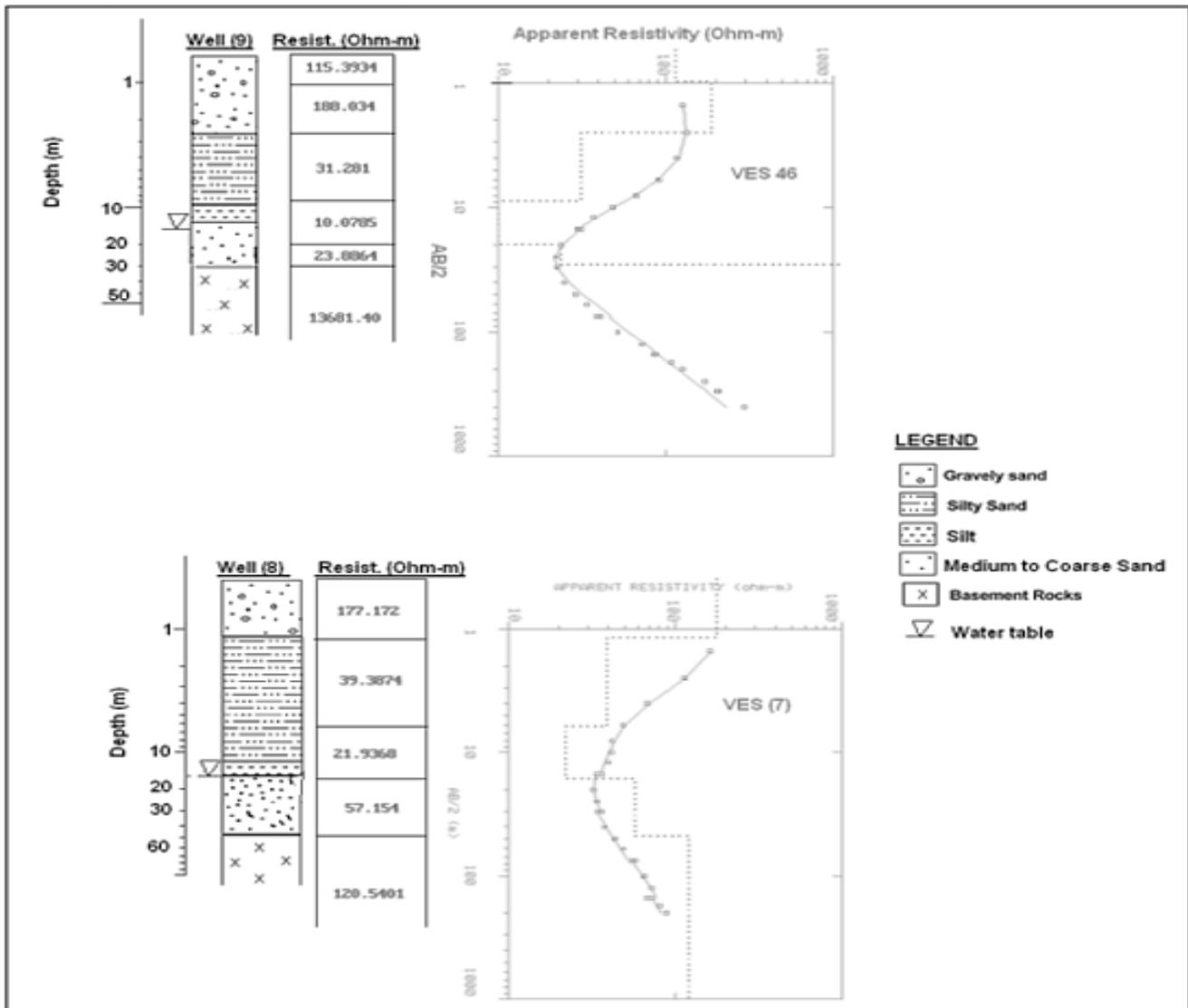
Fig. 5: Interpretation of geo-electric curves compared to borehole lithological logs.
