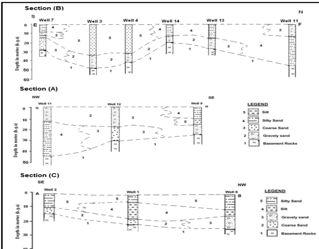
Fig.7: Geological cross-sections.
