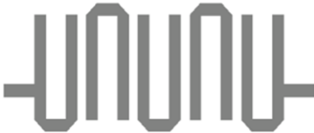
Figure 2.1: tapped line input 5-pole Hairpin Filter
