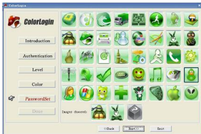
Figure.3: A set of chosen color icons displayed to the user to create pass icons.
