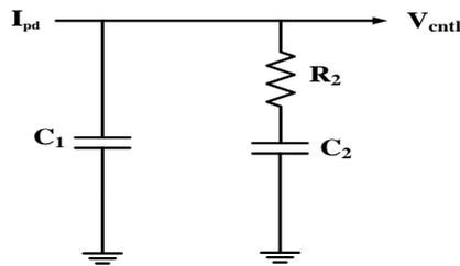
Fig. 14. The 2<sup>nd</sup> order loop filter.
