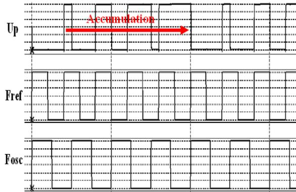
Fig. 3. The simulation results of the digital PFD.
