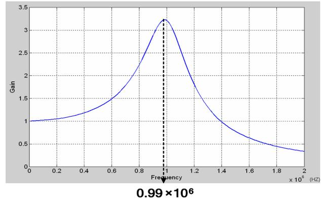
Fig. 15. Gain of PLL with charge pump for  $R_2=100K\Omega$ .
