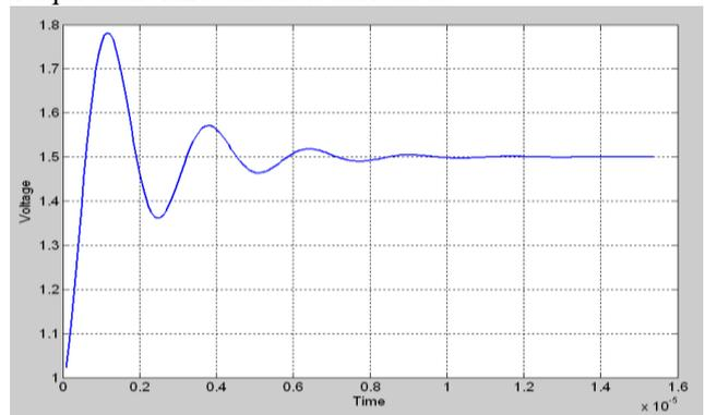
Fig. 7. The output of the 1<sup>st</sup> order low pass filter. ( $R=10\text{K}\Omega$  and  $C=100\text{pF}$ ).
