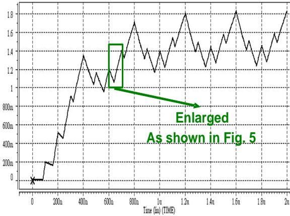
Fig. 4. The HSPICE simulation results of output voltage for the loop filter.
