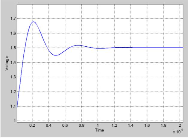
Fig. 11. The output of the low pass filter with zero. ( $R_1=36K\Omega$ ,  $R_2=4K\Omega$ , and  $C=100$  pF)
