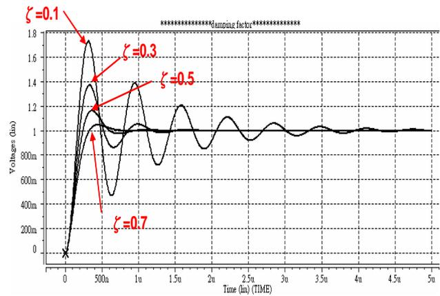
Fig. 9. The results of nonlinear transient analysis with damping factor,  $\zeta = 0.1, 0.3, 0.5$  &  $0.7$ .
