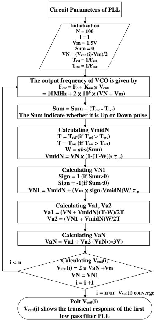
Fig. 12. Calculation flowchart of the regular PLL.
