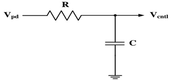
Fig. 6. The 1<sup>st</sup> order low pass filter.
