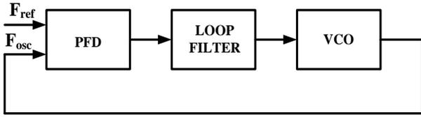
Fig. 1. The basic structure of PLL.
