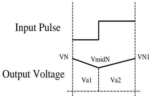
Fig. 5. The output of loop filter within one pulse cycle.
