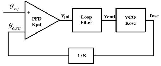
Fig. 2. Linear small-signal model of phase-locked loop.
