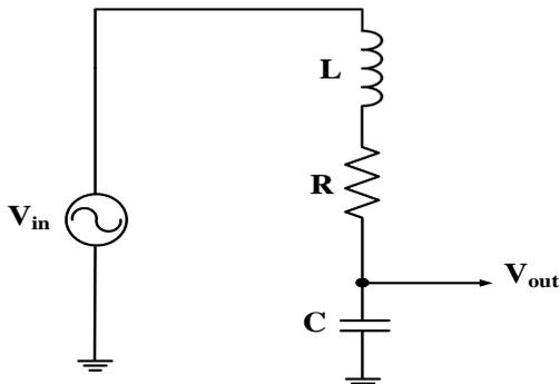
Fig. 8. An equivalent RLC circuit.
