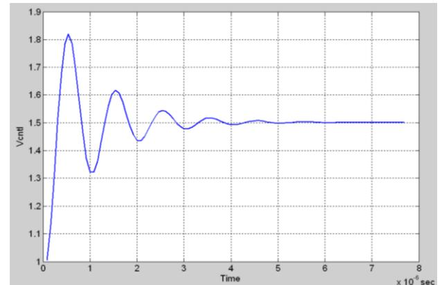
Fig. 16. Result of simulated  $V_{cntl}$  for  $R_2=100k\Omega$ . ( $I_{pd}=100\mu A$  and  $C=50pF$ ).
