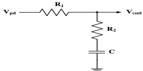
Fig. 10. The 1<sup>st</sup> order low pass filter with zero.
