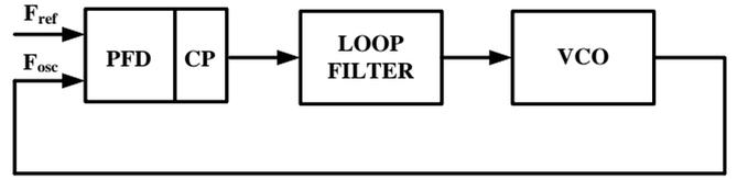
Fig. 13. The basic structure of PLL with charge pump.
