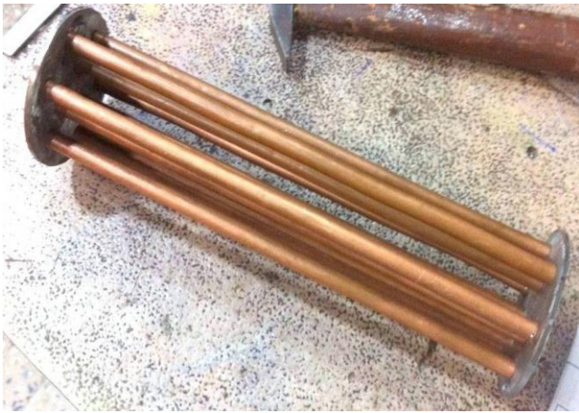
Fig 5 Internal Arrangement of Heat Exchanger to cool Hot exhaust gas into lower temperature T-1=190^{\circ}\text{C} > T-2=75^{\circ}\text{C}
