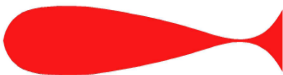
Fig 3. Section of fishtail rudder
