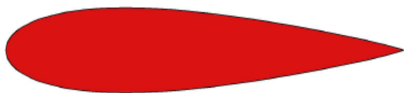
Fig .2. Section of Conventional rudder
