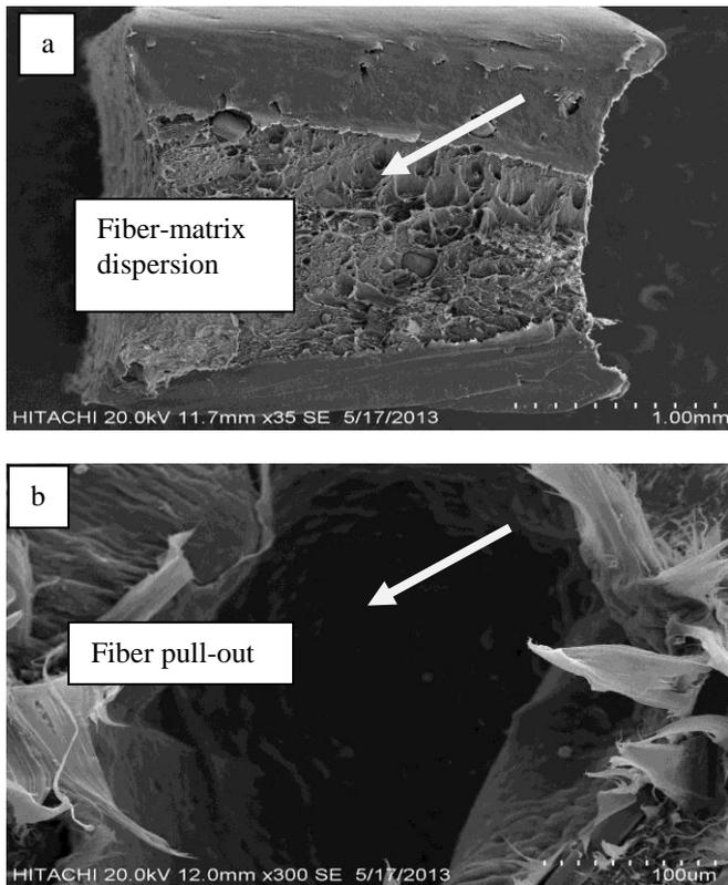
**Fig.4 SEM Fractomicrographs for Samples with Various Fibers loading; (a) 10 % (250  $\mu$ m)**
