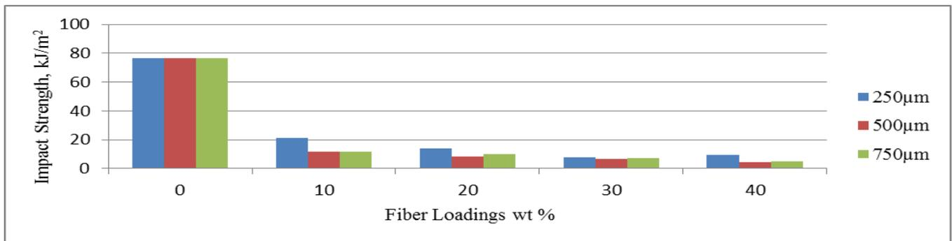
Fig. 3 Impact strength of MH-HDPE composites at various fiber loadings and size
