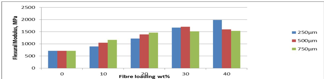
Fig. 2 Flexural modulus of MH-HDPE composites at various fiber loadings and size.
