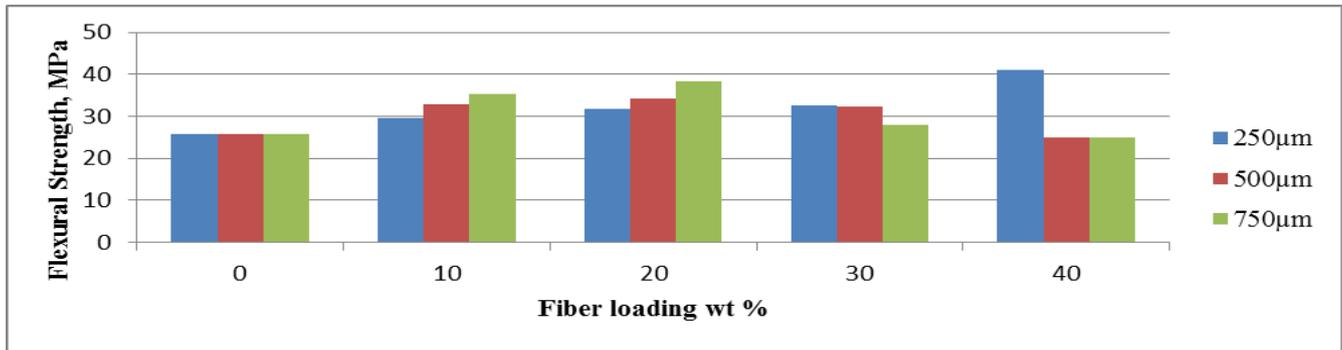
Fig. 1. Flexural strength of MH-HDPE composites at various fiber loadings and size.
