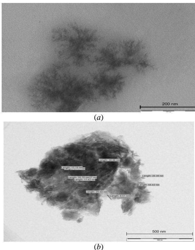
Figure 1. Electron microphotographs of highly branched dendrimeric sol-gel aluminosilicate (a) and of **AIO(OH)** (b) to be placed in between the crowns of the dendrimer ensembles.
