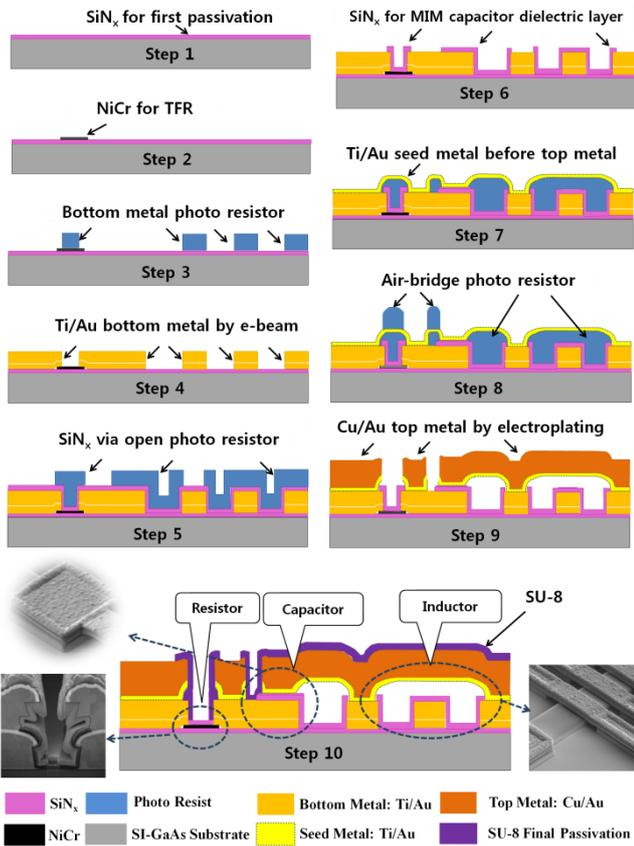
Fig. 4 The optimized IPD fabrication process flow.
