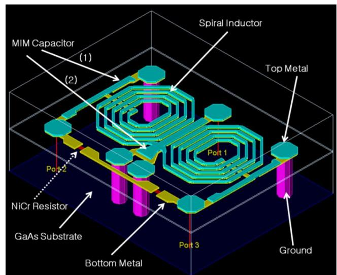
Fig. 2 Three-dimensional (3-D) view of the proposed Wilkinson power divider modeled by Advanced Design System (ADS).
