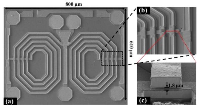
Fig. 8 Focused ion beam (FIB) images of the fabricated IPD Wilkinson power divider: (a) top view, (b) enlarged intertwined air-bridge, and (c) cross-sectional view of the enlarged air-bridge part.
