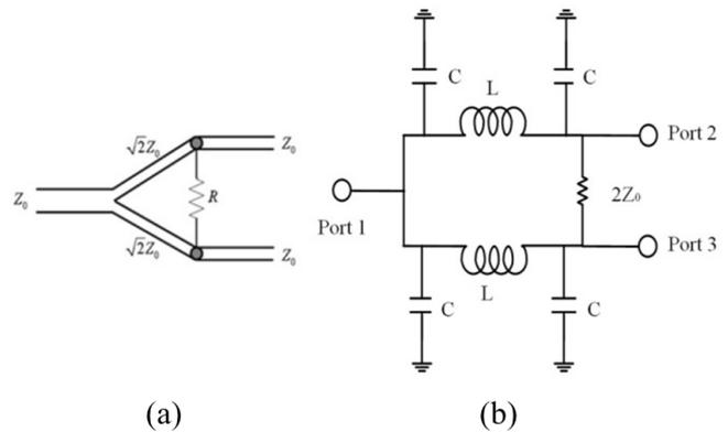
Fig. 1 The schematic structure of: (a) a distributed Wilkinson power divider and (b) a lumped Wilkinson power divider.
