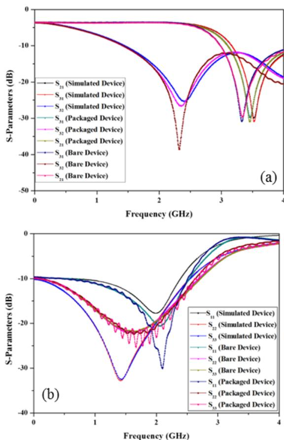
Figure 9. The final S-parameters comparison among the simulated results, measured results of the bare fabricated power divider, and packaged power divider: (a) transmission ( $S_{21}$  and  $S_{31}$ ) and isolation ( $S_{32}$ ) properties and (b) input matching ( $S_{11}$ ) and output matching ( $S_{22}$  and  $S_{33}$ ) performances.
