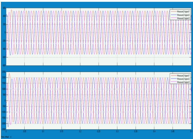
Fig. 15: Constant Output Voltage and Current with 5 th Order Harmonics Input
